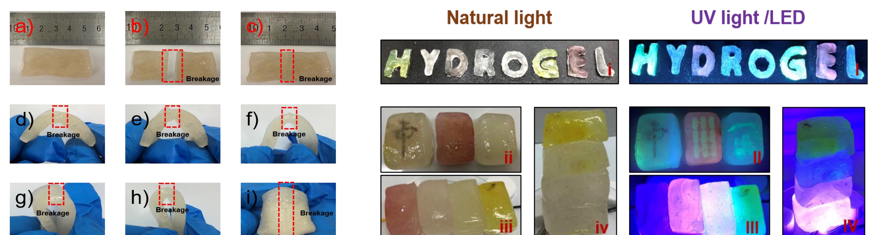
Fig. 9. a) Photo of the initial hydrogel. b) Hydrogel after being cut. c) Hydrogel after self-healing. d-i) Different angles displaying the self-healed hydrogel. Fig. 10. The colour of hydrogel doped with quantum dots of various colours under natural or UV lights (purple LED chip).
